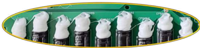
Electrical shock prevention silicon application (front / rear)
