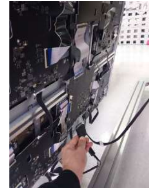
Fig.2 Connect OCM cable
