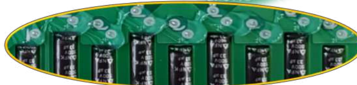
Electrical shock prevention silicon application (front / rear)
