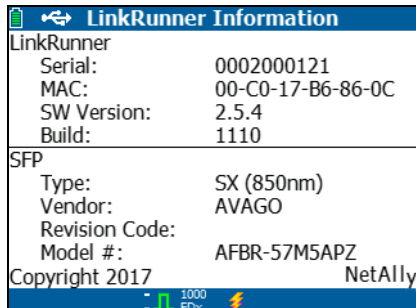
Figure 13. LinkRunner Information Screen with Connected Fiber Adapter
