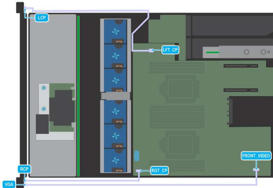
Figure 51. VGA and Control Panel
