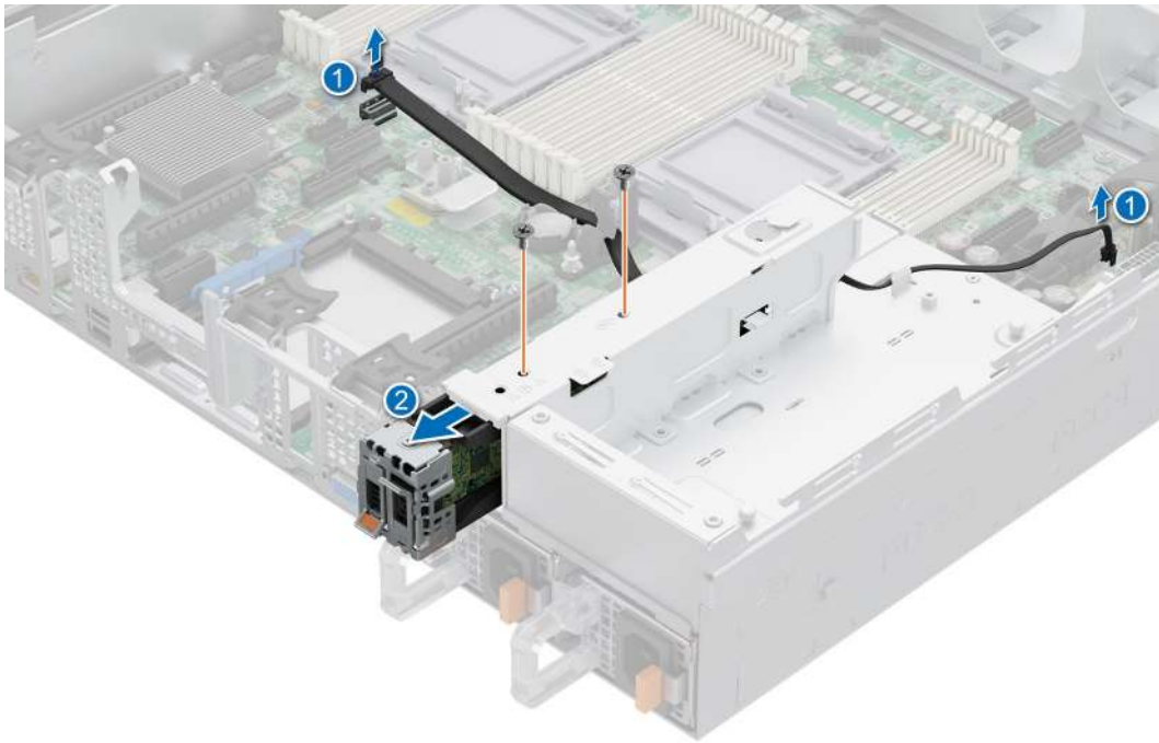
Figure 76. Disconnecting the BOSS power cable and signal cable
