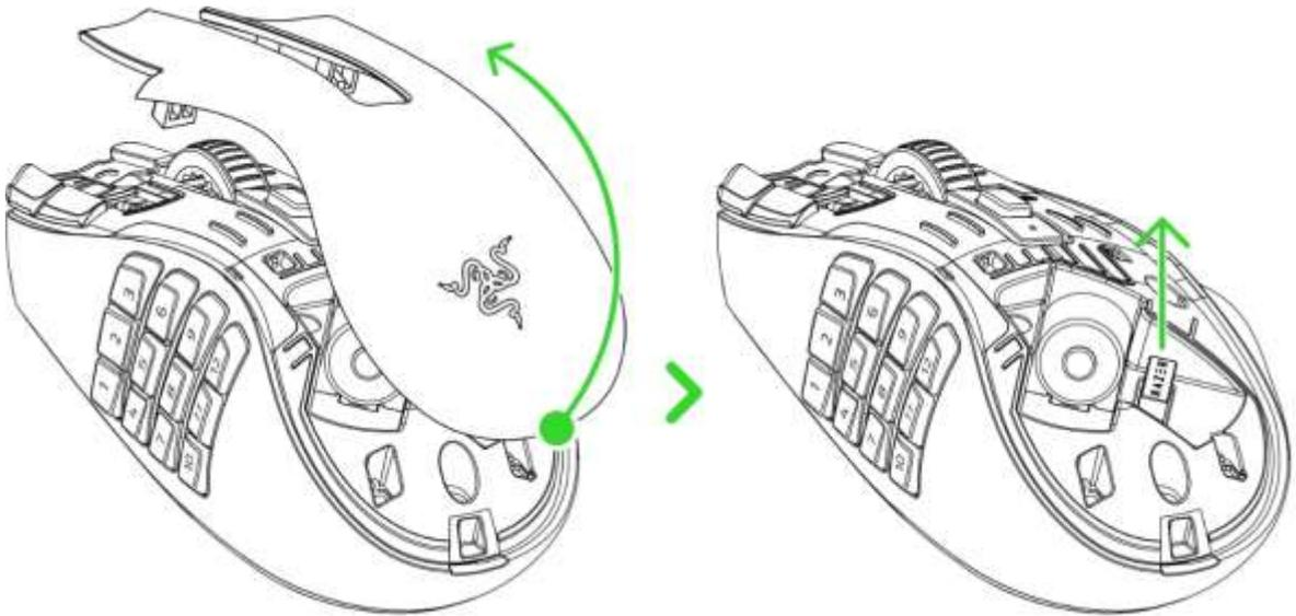
2. Reattach the top cover and plug the wireless USB dongle into your PC.
