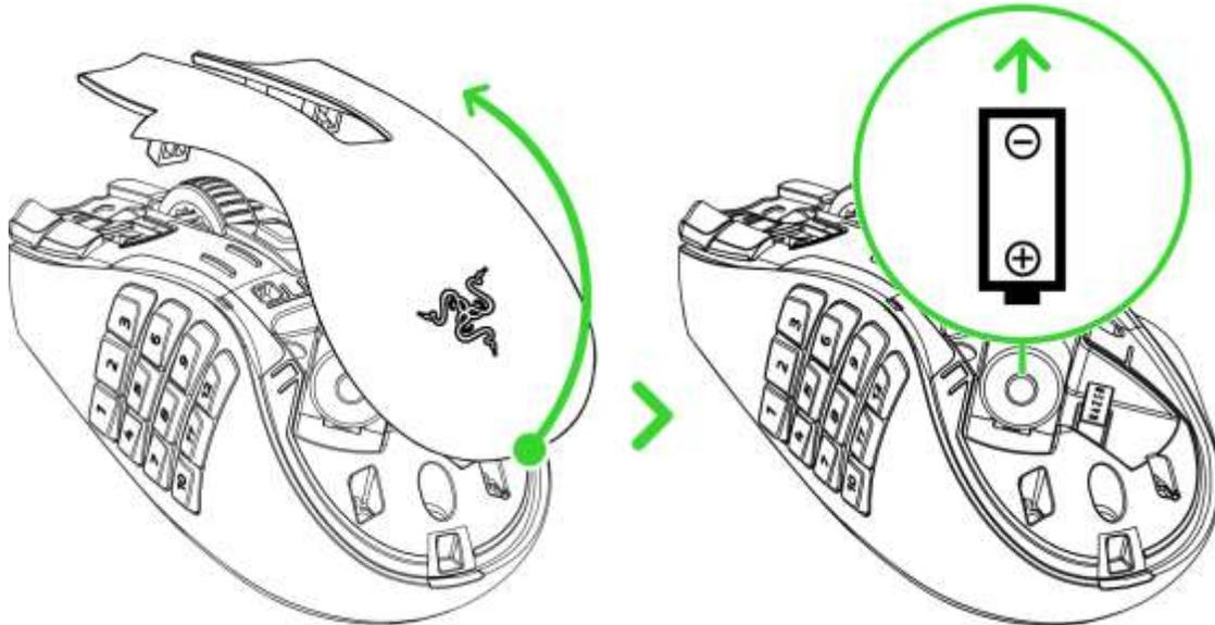
**Caution: The included AA battery is non-rechargeable. Dispose of batteries in accordance with your local environmental laws. For your safety, use only lithium or alkaline batteries.**
