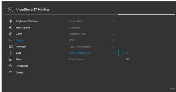
After first synchronization, subsequent syncing is driven by changes to the predefined group of OSD settings from any node in the chain. Any node may initiate the changes downstream and upstream.
