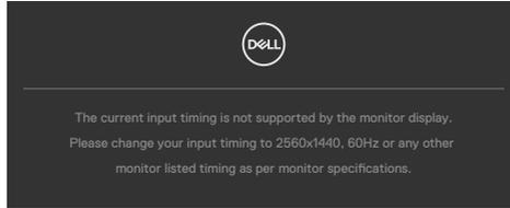
This means that the monitor cannot synchronize with the signal that it is receiving from the computer. See [Monitor Specifications](#) for the Horizontal and Vertical frequency ranges addressable by this monitor. Recommended mode is **2560 x 1440**. You can see the following message before the DDC/CI function is disabled:
