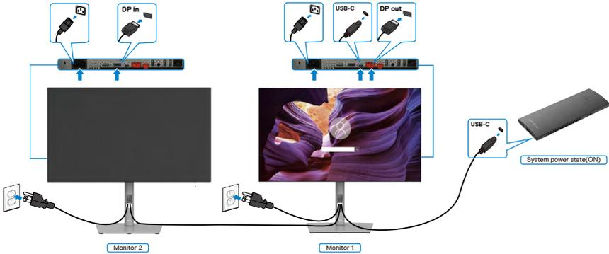
Similarly, a PC is connected to two monitors in an initially ON power state, and the PC system power state is in sync with Monitor 1 power button. When you press the Monitor 1 or PC power button, both the Monitor 1 and PC turns OFF. Meanwhile the Monitor 2 will be in Standby mode. You need to manually press the power button on Monitor 2 to turn it OFF.
