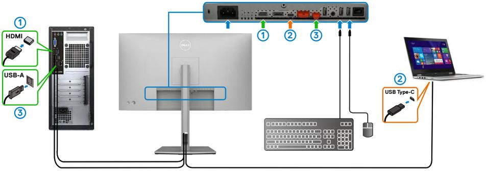
**NOTE:** The USB-C connection currently supports video and data transfer. Ensure **USB Selection** for **HDMI** is set to **USB-C 2**.
