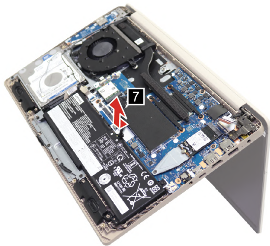
Figure 56. Remove the upper case assembly
