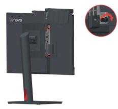
2. Push the computer from the rear as shown to disconnect it completely from the 3 in 1 cable.
