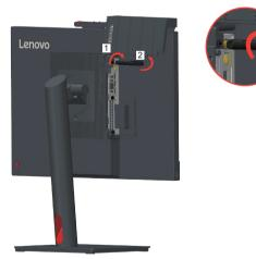
3. Pivot the cable cover as shown to the closed position.
