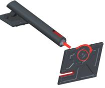
3. Insert the two metal tabs on the stand into the corresponding holes on the rear of the monitor. Then, pivot the stand downward until it clicks into position.
