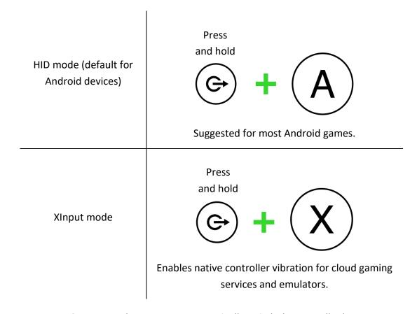
The Razer Nexus Game Launcher app can automatically switch the controller between HID and XInput mode when launching vibration compatible games.
