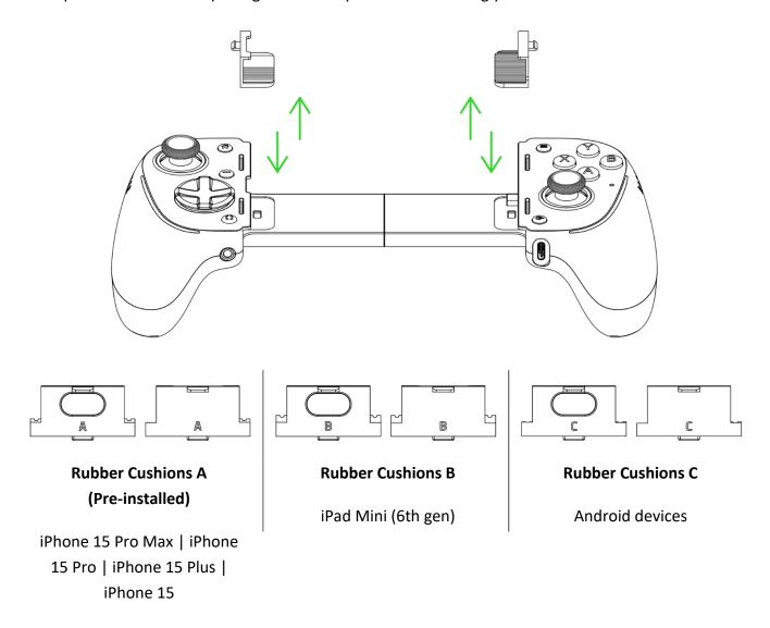
By default, rubber cushions A are pre-installed with the controller. For a case-fitted phone, you can also try removing the rubber cushions to see if it's compatible with the controller.
