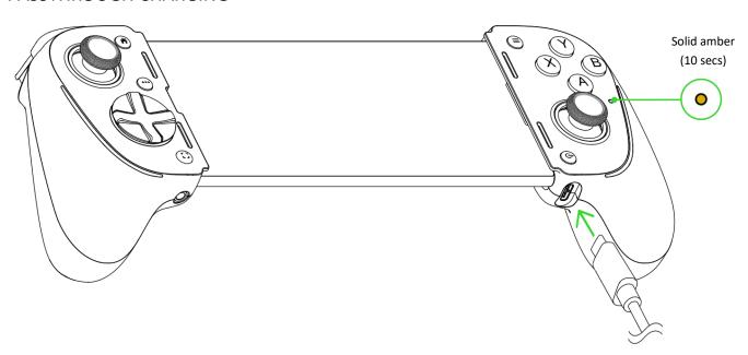
When using the passthrough charging feature, the status indicator will briefly display a solid amber status. Make sure to only use a USB-IF-certified charging cable. USB Type C audio and other accessories are not supported.
