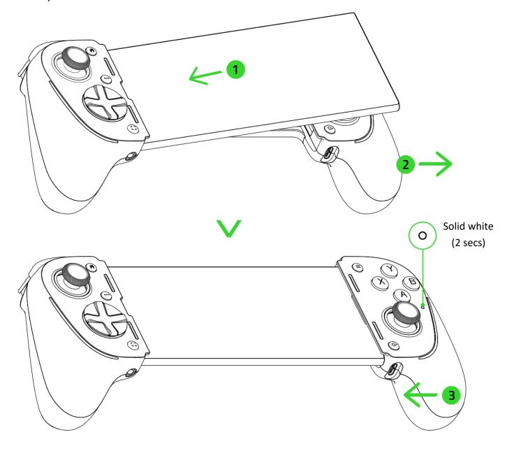
The controller can support maximum device dimensions of 12.32 mm (thickness, including camera) x 208.9 mm (Length) for phones and tablets.
