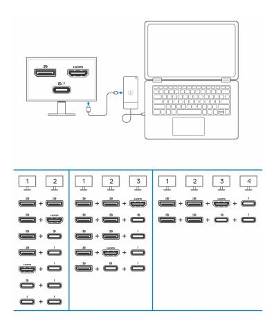
The above table shows the different video port combinations available to connect multiple displays to the Dell WD22TB4 dock. For more details on supported display resolutions, please see Display Resolution.
