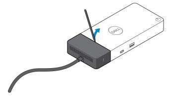
**4.** Gently wiggle and remove the USB Type-C cable module from its connector on the docking station.
