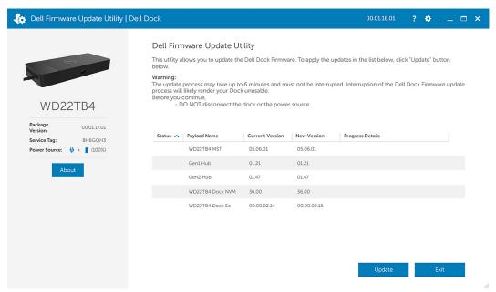
3. Wait for all the component firmware update to complete. A progress bar is displayed in the bottom.
