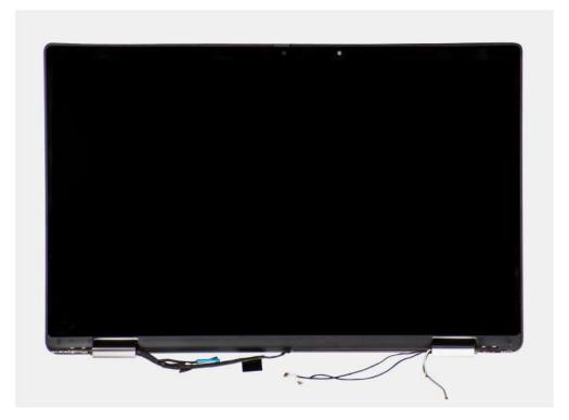
Figure 1. Display assembly with antennae cables
