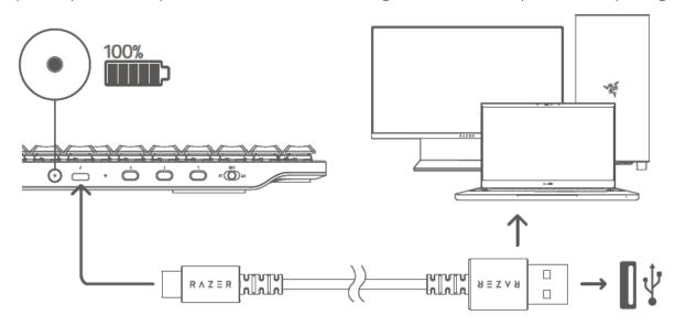
For best results, fully charge your keyboard before using it for the first time. It takes approximately 2 hours to fully charge your keyboard. You may continue using the keyboard while plugged in.
