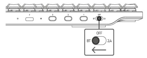
2. Up to 3 Bluetooth devices can be paired and registered to your keyboard (one for each profile). To activate the pairing mode of your preferred profile, press and hold its corresponding button for 5 seconds. The numerical key on your keyboard will then light up to show which profile has been activated.
