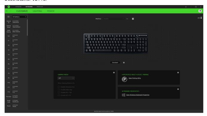
Alternatively, you can skip to a specific key assignment by selecting it on the Customize tab.
