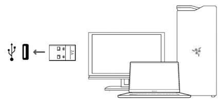
Use the wireless USB extender and Type A to Type C cable to increase the reach of your 2.4GHz wireless USB dongle if the signal is weak, intermittent, or out of range.
