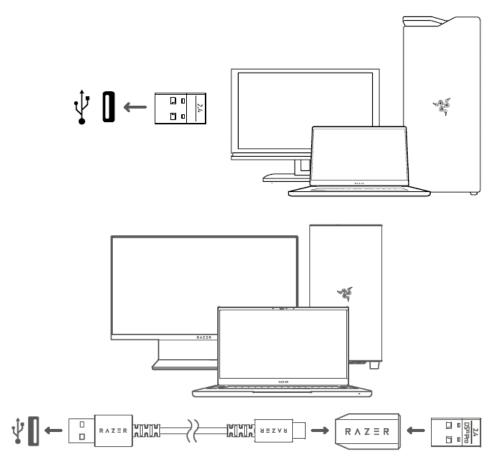
If you have a compatible Razer device with 2.4GHz wireless connectivity, you can do a multi-device pairing and use the same dongle for both devices. Visit this link to learn more about multi-device pairing: <a href="https://rzr.to/NAV6x0">https://rzr.to/NAV6x0</a>
