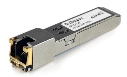
The SFPC1110 is a Cisco SFP-GE-T compatible copper transceiver module that has been designed, programmed and tested to work with Cisco® brand switches and routers. It delivers dependable 1GbE (1000 Mbps) connectivity over copper cable, for 1000BASE-T compliant networks, with a maximum distance of up to 100 m (328 ft).
