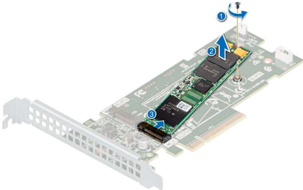
Figure 41. Removing the M.2 SSD module
