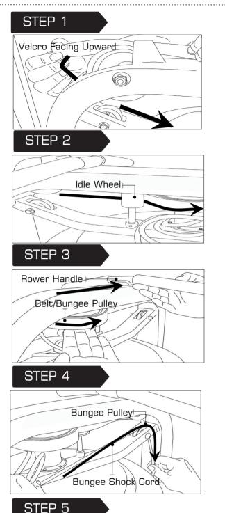
Begin reattaching the Rower Belt by threading around the Rower Belt Pulley with the Velcro side facing upward as illustrated.
