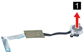
Figure 30. Remove the fingerprint board lens light guide
