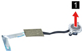
Figure 73. Remove the fingerprint board lens light guide
