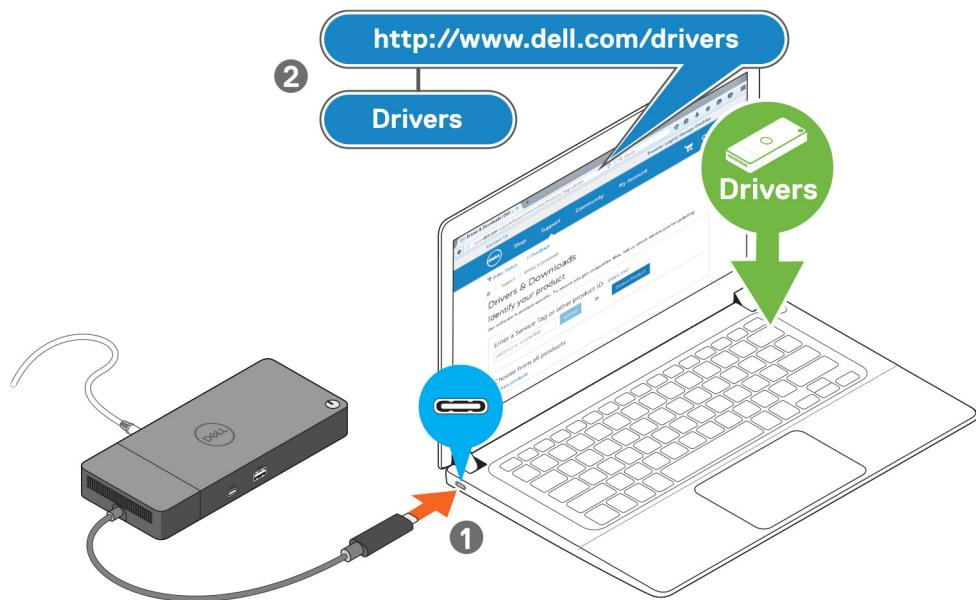
**Figure 7. Connecting the USB Type-C connector**
