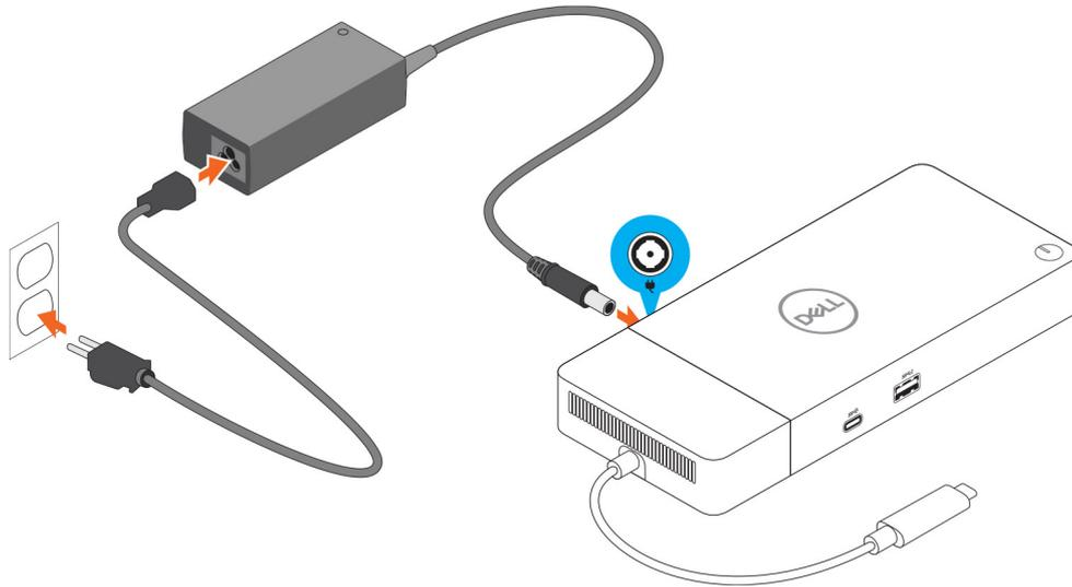
**Figure 6. Connecting the AC Adapter**
