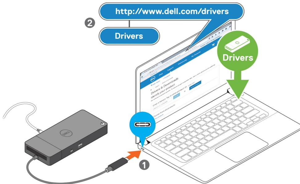
**Figure 7. Connecting the USB Type-C connector**
