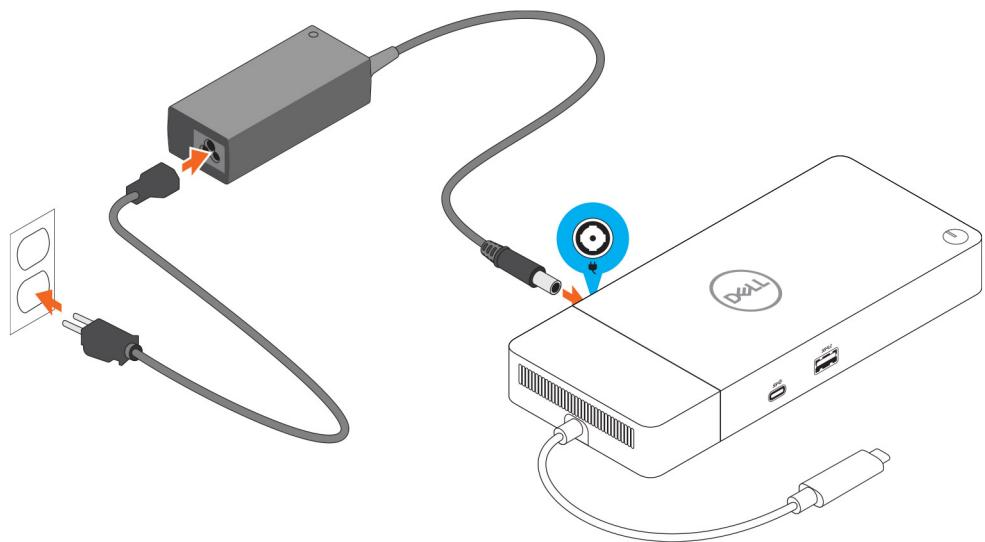
**Figure 6. Connecting the AC Adapter**
