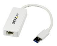
The USB31000SPTW USB 3.0 to Gigabit Ethernet Adapter lets you add a Gigabit network port to your Macbook® or Ultrabook™ computer through a USB 3.0 port, and features an integrated USB 3.0 pass-through port that keeps your USB port available for use with other peripherals. Each RJ45 port supports 10/100/1000 Mbps Ethernet and is fully compatible with IEEE 802.3i/u/ab standards.
