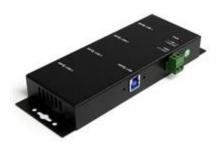
The ST4300USBM Mountable 4-Port Industrial USB Hub (USB 3.0) offers a simple way to expand a systems current USB capability by providing 4 additional external USB 3.0 ports from a single USB 3.0 host connection, with speeds up to 5 Gbps.
