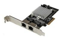
The ST2000SPEXIPCI Express Dual Port Gigabit Network Card lets you add two gigabit Ethernet ports to a desktop computer through a single, four-lane (x4 or higher)PCI Express slot. Each port is fully compatible with IEEE 802.3/u/ab standards, for 10/100/1000 Mbps auto-negotiation.
