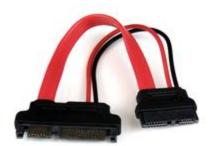
The SLSATAADAP6 Slimline SATA to SATA adapter features a Slimline Serial ATA connector on one end and a standard SATA data connector (with SATA power connector) on the other, enabling you to connect a Slimline SATA optical drive to standard motherboard and power supply connections.
