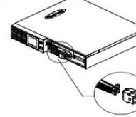
5. Install the replacement batteries by connecting the red and the black wire to the same color wires from the battery pack. Recharge the unit for at least 8 hours to ensure the UPS performs expected runtime.
