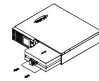
4. Install the new battery pack. Assemble the screws, cover, cable and front panel in the reverse sequence of above steps.
