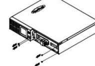
2. Remove four screws from battery compartment cover and remove the cover completely off the unit.
