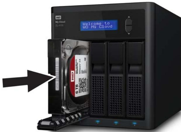
3. Using some force, snap the drive handle shut.
