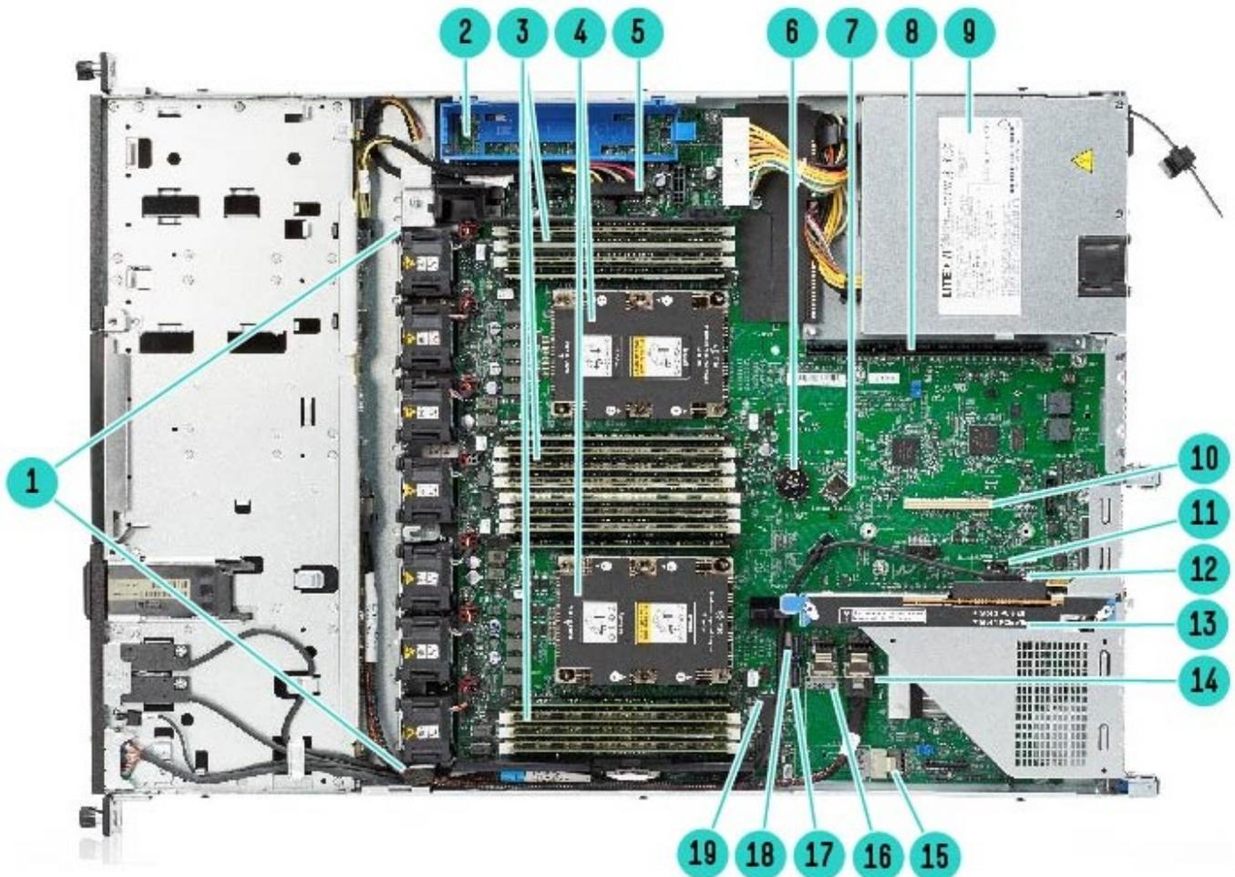
8SFF chassis – with optional 2<sup>nd</sup> CPU - Internal View
