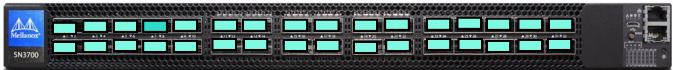
All 32 QSFP56 ports 1-32 support x4 or x2 breakout
