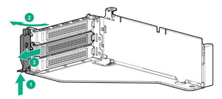
**13.** Install the GPU into the riser.
