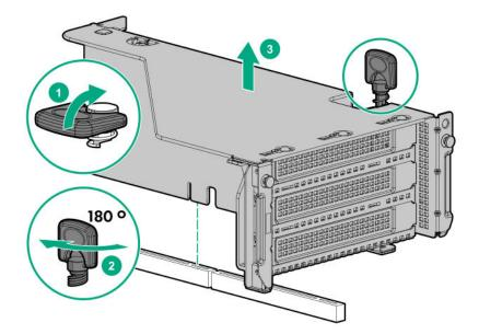
6. Identify and then remove the PCIe blank from the riser cage.
