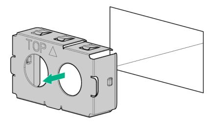
**3.** Insert the power supply into the power supply bay until it clicks into place.
