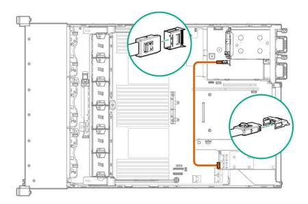
Cable routing: Rear 3LFF SAS/SATA drive option for system board
