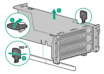
6. Remove the rear wall blank.
