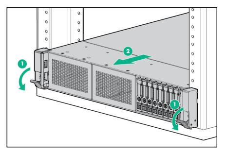
**3.** After performing the installation or maintenance procedure, slide the server back into the rack, and then press the server firmly into the rack to secure it in place.
