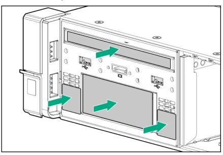
• If the 2SFF drive cage is not installed, then install airflow labels as shown.
