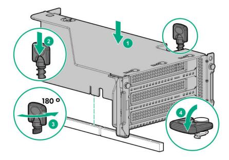
To install the riser in the secondary position, install the secondary riser cage.
