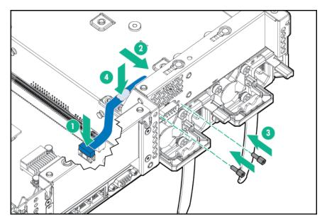
Be sure to remove the backing from the double-sided tape.
