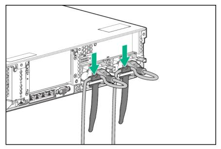
6. Secure the cables to the cable management arm.
