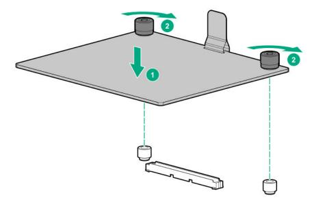
• For Type-p Smart Array controllers, install the controller into an expansion slot.
