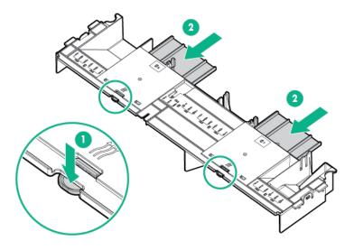
8. Install the appropriate retention clip onto the air baffle.Install the clip that supports your configuration. Primary, secondary, and tertiary positions are shown.
