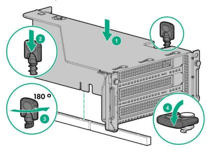
**17.** Slide the retention clips to the locked position.
