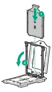
When fully inserted, you will feel the carrier frame engage into the rail frame.
