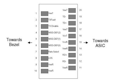
Pin-out of connector Block on Host board
