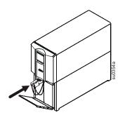
Insert the battery connector into the battery jack and push firmly. A snap will be felt as the connector partially engages the jack. A second snap will be felt as the connector securely seats in the battery jack.
