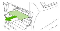
7. If you can see the jammed media, but neither the leading edge nor the trailing edge is visible, gently pull on the sides of the sheet of media until one edge becomes free. Then carefully pull the jammed media out of the fuser.
