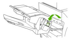
**5.** Close the staple-cartridge cover, and slide the stapler/stacker into the MFP.
