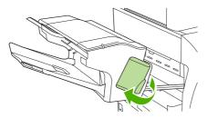
4. To remove the staple cartridge, pull up on the green handle and pull out the staple cartridge.
