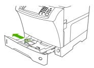
3. Press the tab on the front media guide and slide the guide all the way out.
