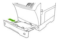
6. Adjust the front media guide by pressing the tab on the guide and sliding the guide until it gently touches the media stack.
