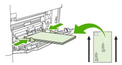
3. Adjust the guides to touch the envelope stack without bending the envelopes. Make sure that the envelopes fit under the tabs and maximum-height indicators on the guides.
