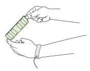
6. Hold the DIMM by the edges, and align the notches on the DIMM with the DIMM slot. (Check that the locks on each side of the DIMM slot are open.)
