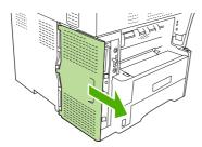
**4.** If necessary, remove the plastic fax-accessory cover from the formatter. Insert a coin into the groove at the top of the cover, and use it to pry the cover away from the formatter.
