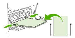
For tray2 and the optional 500-sheet trays, load paper with the front side facing down, and the top, short edge toward the right.
