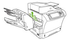
4. If the jammed media is inside the 3-bin mailbox or the stapler/stacker, carefully pull the jammed media up and out of the device.
