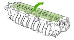
11. Reinstall the fuser. Push on the fuser with your thumbs to be sure it snaps securely into place.
