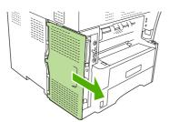
4. Open the formatter-cage door by grasping the metal tab and pulling the door open.
