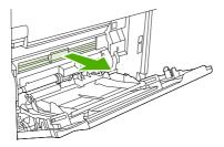
**5.** Rotate the paper-release guide to check for additional jammed media underneath. If jammed media is present, remove it.
