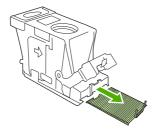
7. Close the lever at the back of the staple cartridge. Be sure that it snaps into place.
