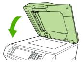
5. Pull the release lever to open the document-feeder cover.
