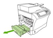
3. Check for jammed paper in the optional duplexer. Carefully pull out the jammed paper.
