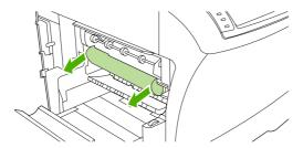
**8.** If the media tears as you are removing it, turn the green dial on the fuser, and then carefully pull out the jammed media. Go to step 13.
