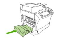
**14.** Reinstall the output-bin assembly, the 3-bin mailbox, or the stapler/stacker. Insert the device at an angle, and then slide it into the device.
