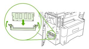
7. Press the DIMM straight into the slot, and press firmly. Make sure the locks on each side of the DIMM snap into place.
