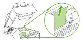
**4.** If jammed media is difficult to remove, open tray 1 and remove the envelope-entrance cover. If media is present, remove it.
