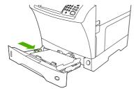
**4.** Adjust the media-width guide by pressing the tab on the guide and moving it until it touches the media stack.
