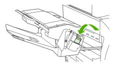
9. Close the staple-cartridge cover, and slide the stapler/stacker into the device.
