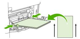
For tray2 and the optional 500-sheet trays, load the paper with the front side facing down, and the top, short edge toward the right.
