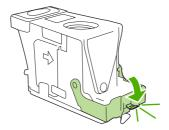
8. Reinsert the staple cartridge into the staple-cartridge holder, and push down on the green handle until it snaps into place.
