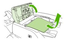
3. Lift the green jam lever on the document guide, and then check for jammed media. Carefully remove any jammed media.
