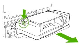
3. Slowly remove any jammed envelopes from the optional envelope feeder and from the device.
