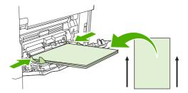
10. Make sure the media fits under the tabs on the guides and not above the load level indicators.
