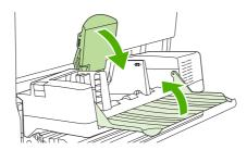
2. Press and hold the release button on the left side of the optional envelope feeder. Grasp both sides of the optional envelope feeder and carefully pull it out of the device.
