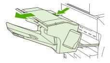
2. If you are using a 3-bin mailbox or a stapler/stacker, remove any media that is stacked, and then press and hold the release button on the top of the accessory. Slide the accessory away from the device.
