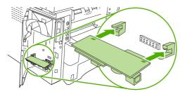
**9.** Push the fax accessory into place, and then verify that it is securely connected to the formatter. The phone connector on the fax accessory should be aligned with the square opening in the formatter cage.
