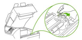
3. Slowly pull any jammed media out of the device. Do not tear the media. If part of the sheet has already been pulled into the device, follow the steps for <u>Clear jams from the top-cover and print-cartridge areas</u>.
