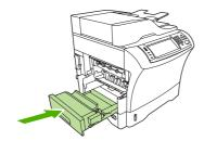
7. Reinstall the output bin (or reinstall the 3-bin mailbox or the stapler/stacker).
