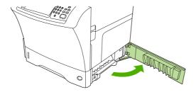
2. Carefully pull out any jammed media from either the top or the bottom of the jam-access area.
