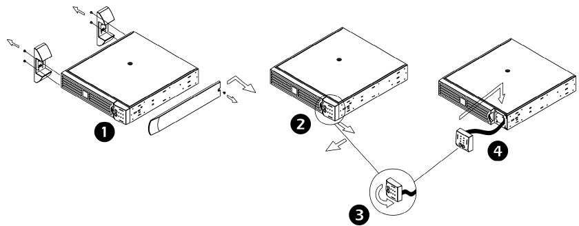
If using a rack-mount configuration, begin here. NOTE: Cleats will be factory installed on units purchased for rack-mount configuration.
