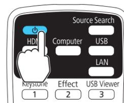
**Note:** To shut down the projector, press the power button twice.
