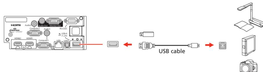
If you connect a digital camera, USB flash drive, or USB storage device, you can use the projector's PC Free feature. See the online *User's Guide* for details.
