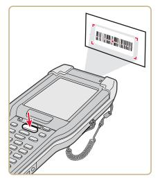
For near or close-in scanning distances of 30 cm (11.8 in) or less, use the laser pointer as a guide and aim slightly to the right of the center of the bar code. Make sure the illumination beam covers the bar code you are trying to decode.
