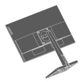
Step 4: Attach the mounting bracket from the VESA compatible wall mounting kit (100mm  $\times$ 100mm distance), VESA Mounting Screw M4  $\times$  10 mm.
