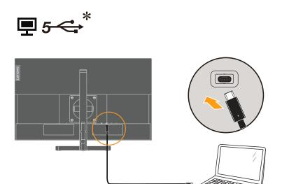
7. Connect one end of the USB cable to the USB downstream terminal of the monitor, and connect the other end of the USB cable to an appropriate USB port on your device.
