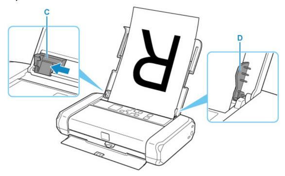
**5.** Slide the paper guide to align it with the paper stack.
