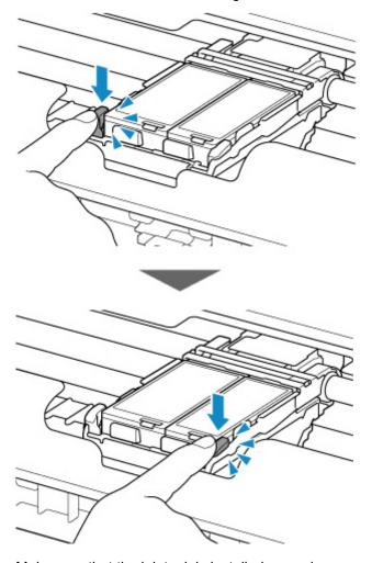
Make sure that the ink tank is installed properly.
