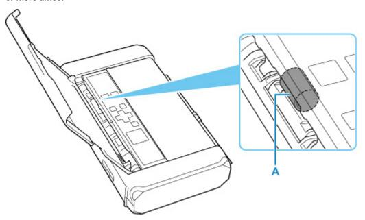
After cleaning the paper feed roller with a cotton swab, turn on the power, then clean the paper feed roller again.
