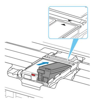
6. Press the PUSH mark on the ink tank until the ink tank snaps firmly into place.
