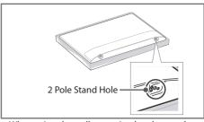
When using the wall mounting bracket, apply the adhesive protective label or protective cover to cover the unused stand openings. This will prevent the accumulation of dust and dirt. (Use only when provided with your particular model.)
