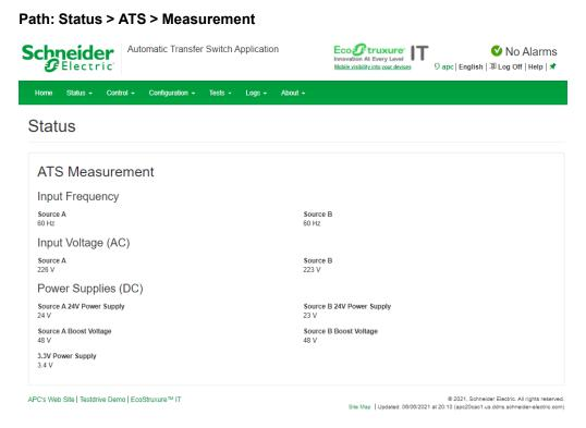
View measurements for Input Frequency, Input Voltage (AC), and Power Supplies (DC).
