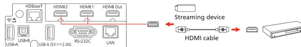
**Note:** If you connected a streaming device to an HDMI port, you can also connect it to the projector's **USB-A** (flat) port for power.
