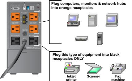
3. Plug the PowerSure PSA's attached 6-ft. (1.8m) power cord into an AC outlet. Check that the Site Wiring Fault Indicator on the rear is not illuminated. If it is lit, refer to the **Troubleshooting** section.
