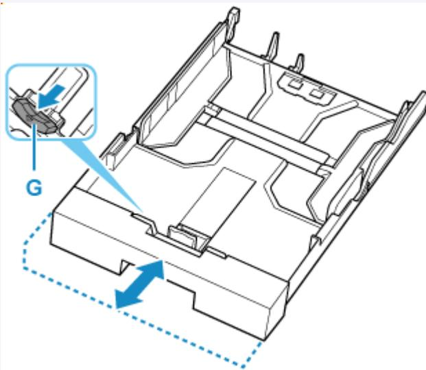
**4. Move the paper guide and adjust the guides to edge of the paper stack.**
