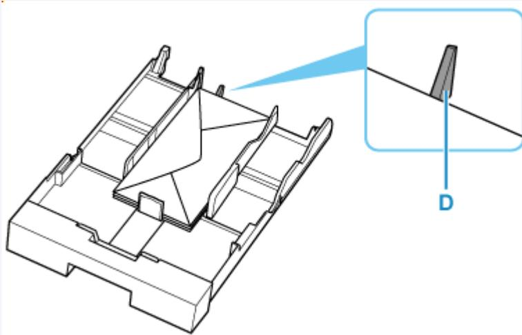
4. Move the paper guide and adjust the guides to edge of the paper stack.
