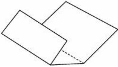
9. Load only this sheet of paper in the cassette with the ridges of the creases facing up and the edge of the half with no crease facing to the far side.
