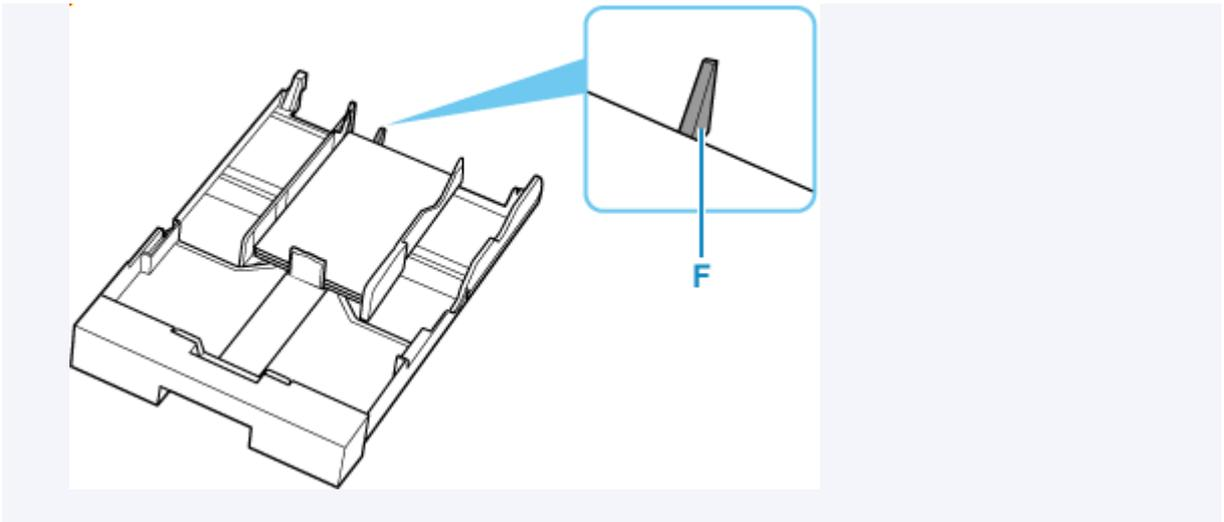
**4.** Move the paper guide and adjust the guides to edge of the paper stack.
