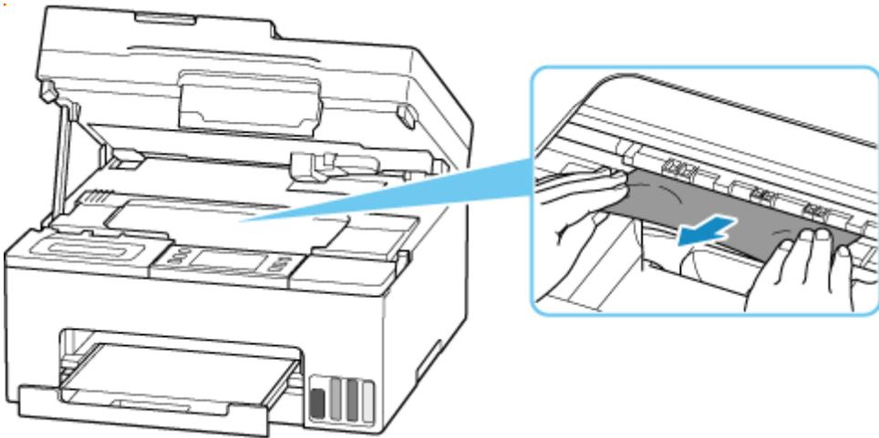
If the paper is rolled up, pull it out and grasp the edges of the paper.
