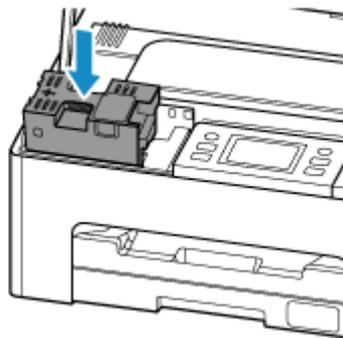
**9.** Slide the maintenance cartridge to the right until it reaches the end.
