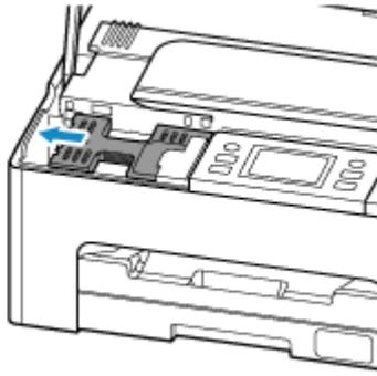
7. Lift the maintenance cartridge and remove it.
