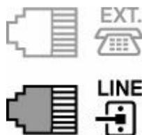
When you connect the telephone to the printer, make sure that the printer is turned off, connect one end of the modular cable to the external device jack near the "EXT." mark of the printer, then connect the other end to the telephone line jack of the telephone.
