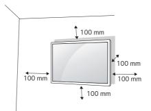
To install your monitor on a wall, attach a wall mounting bracket (optional part) to the back of the monitor. Make sure that the wall mounting bracket is securely fixed to the monitor and to the wall.
