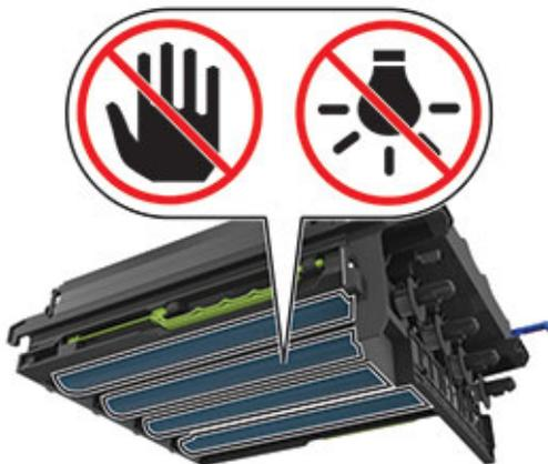
9. Insert the imaging unit tray until it is fully seated.
