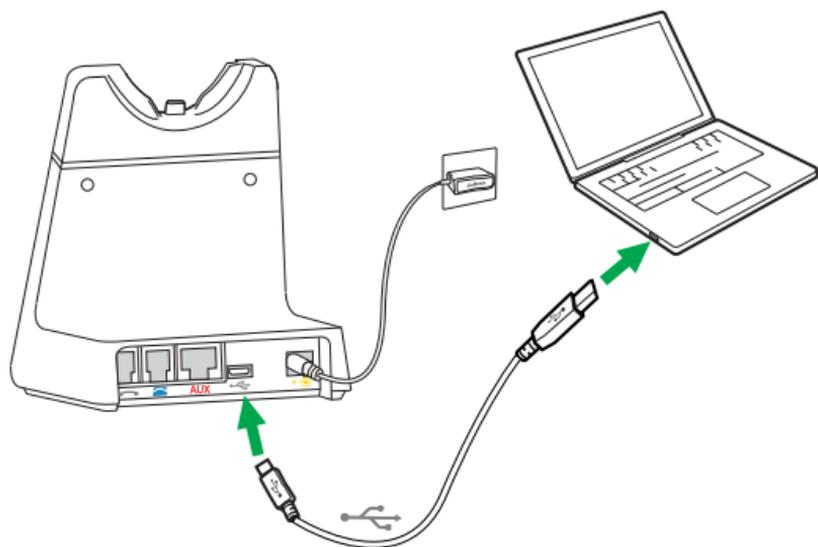
1. Plug the supplied micro-USB cable into the port marked
