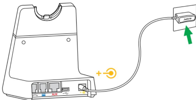
Plug the base into a power supply using the supplied power cable.
