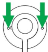
The convertible headset uses a motion sensor to detect which button is volume up and which is volume down, depending on the headset orientation
