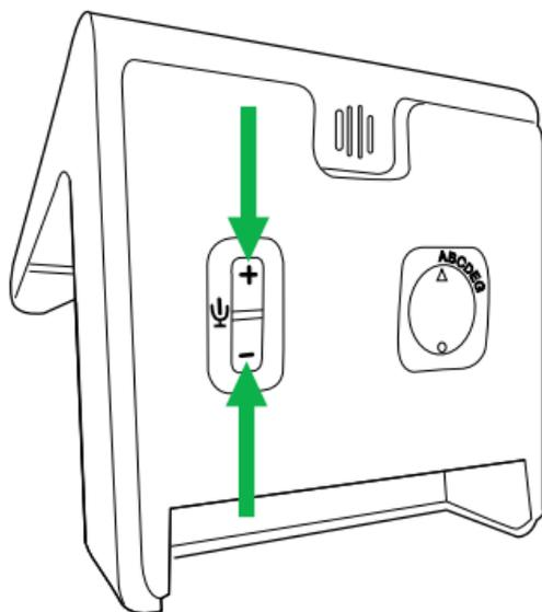
To adjust the desk phone microphone volume, press  $+$  or  $-$  buttons, located on the bottom of the base.
