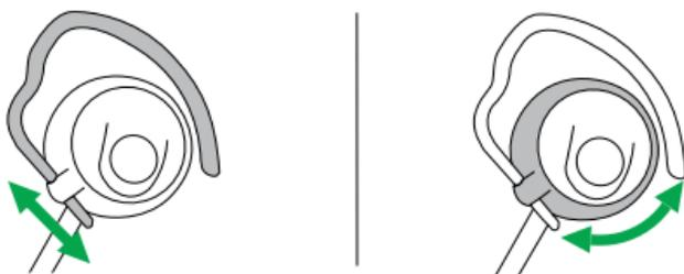
The EarHooks are flexible, and can be bent to suit your ear for a secure and comfortable fit.
