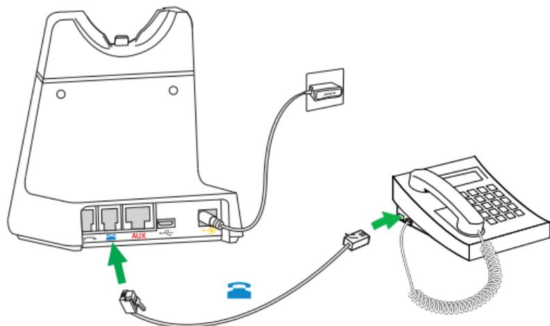
1. Plug the supplied telephone cable into the port marked
