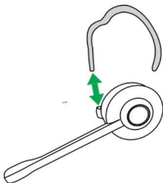
The EarHook with one dot is the medium size, and the EarHook with two dots is the large.
