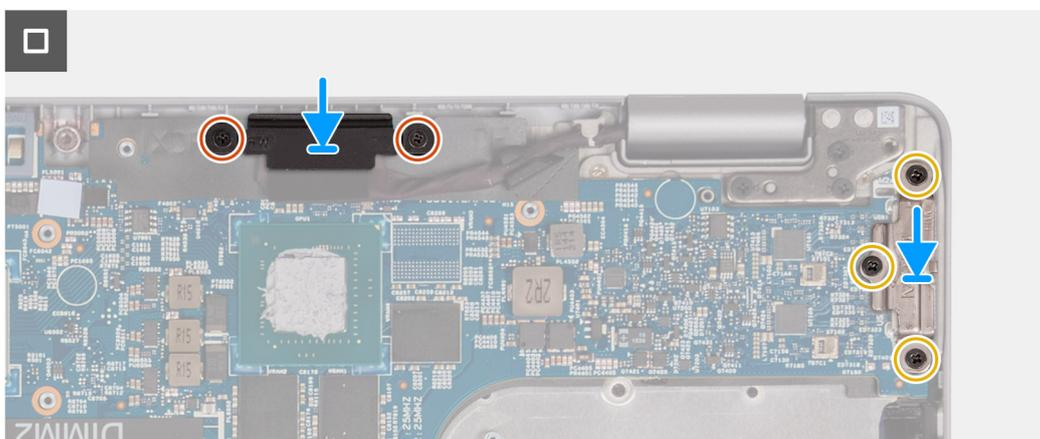
**Figure 64. Installing the system board**
