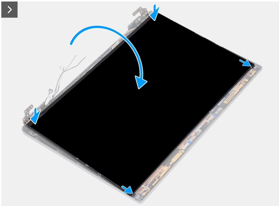
Figure 86. Installing the display panel
