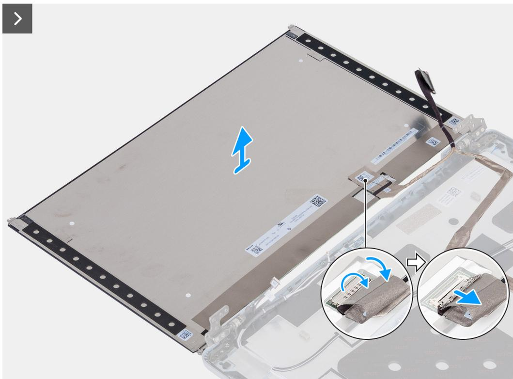
Figure 82. Removing the display panel
