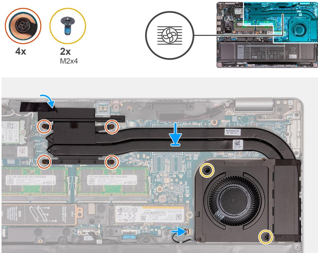
**Figure 55. Installing the fan and heat-sink assembly (Integrated GPU)**
