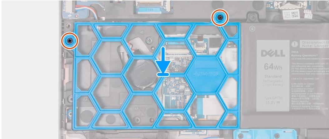
Figure 36. Installing the 4-cell battery plastic filler
