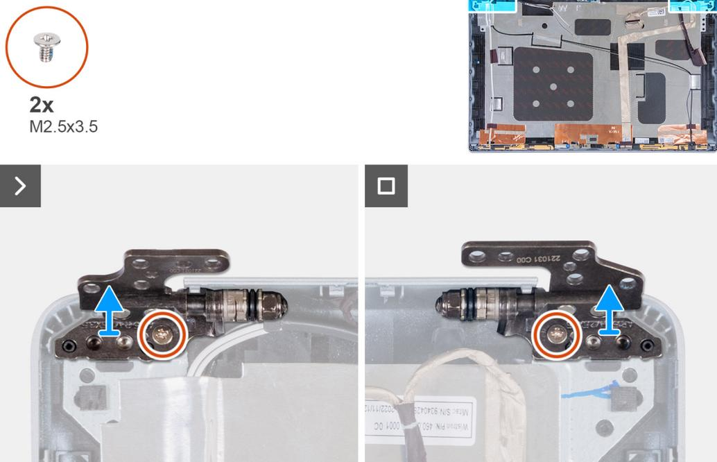
**Figure 90. Removing the display hinges**
