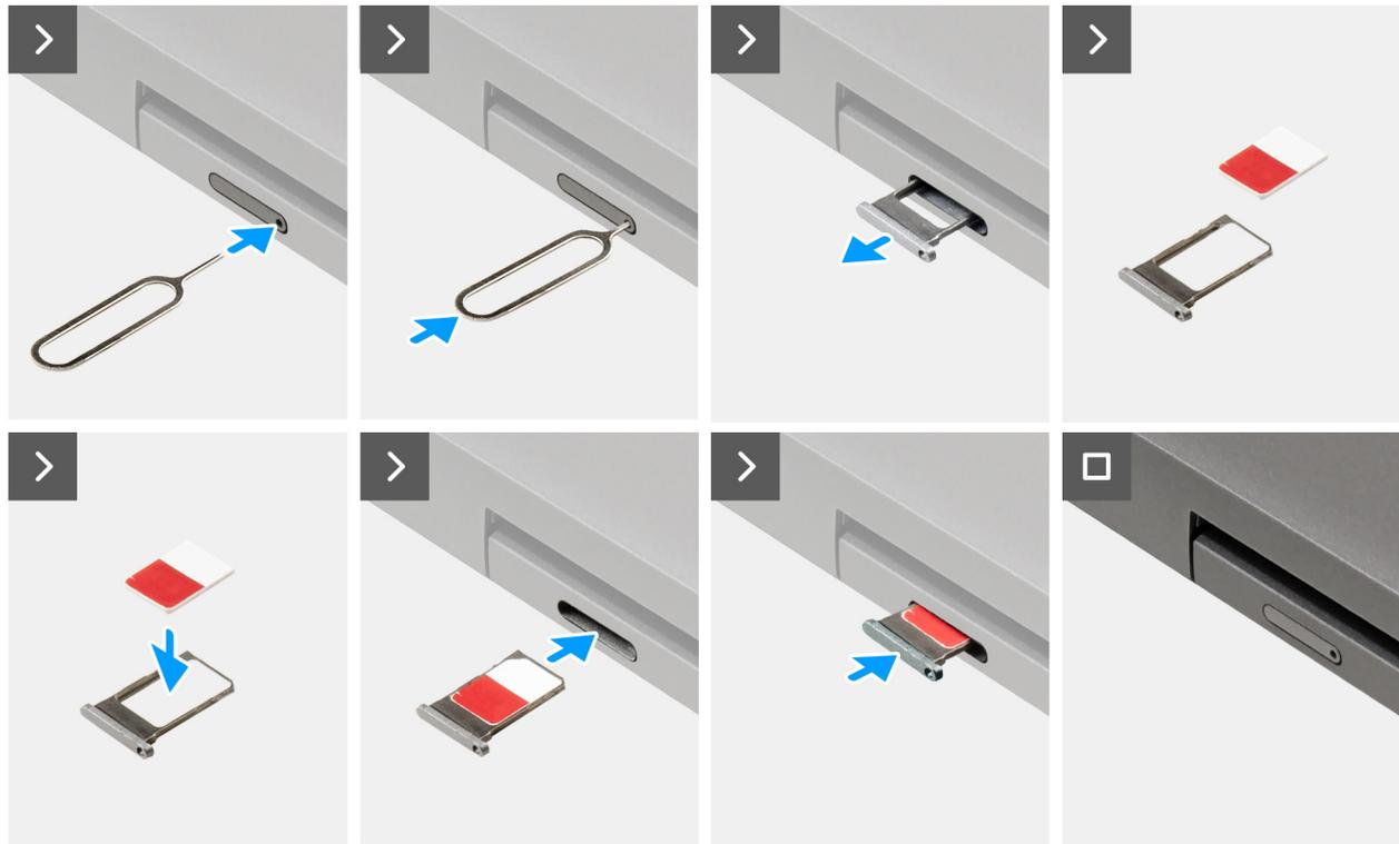
Figure 12. Installing the SIM card tray
