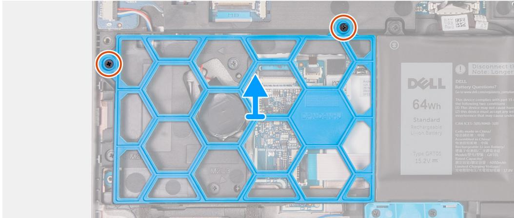
Figure 35. Removing the 4-cell battery plastic filler
