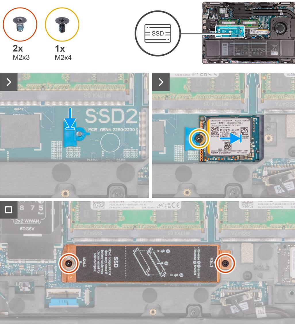
**Figure 32. Installing the M.2 2230 SSD in slot 2**
