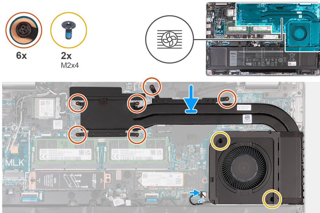
**Figure 53. Installing the heat sink (Discrete GPU)**
