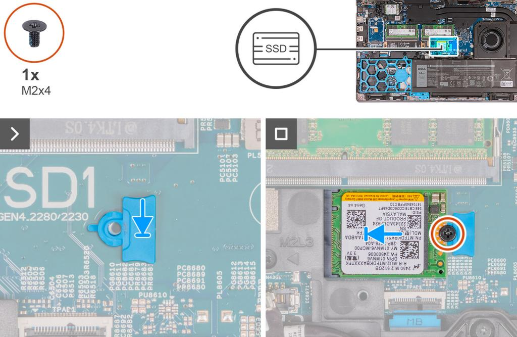
**Figure 28. Installing the M.2 2230 SSD in slot 1**
