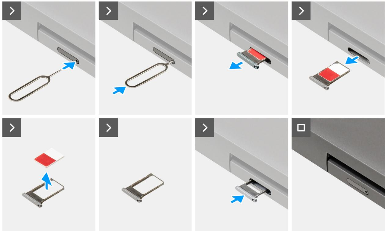
**Figure 11. Removing the SIM card tray**
