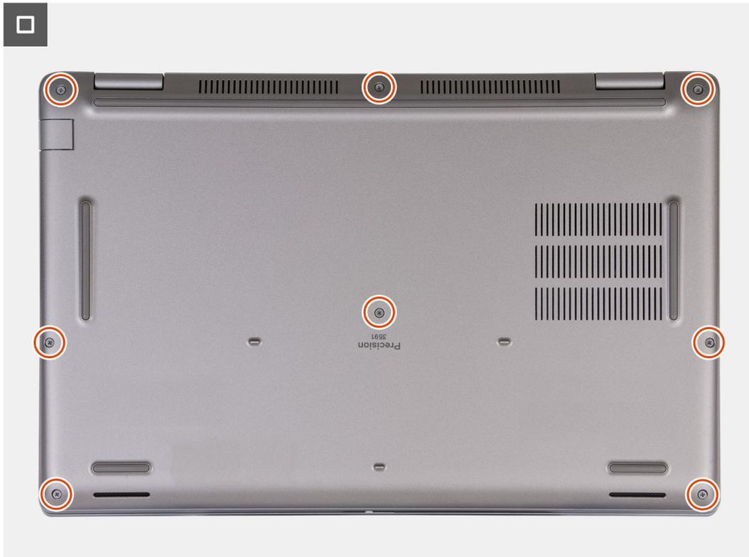
**Figure 18. Tighten the captive screws**
