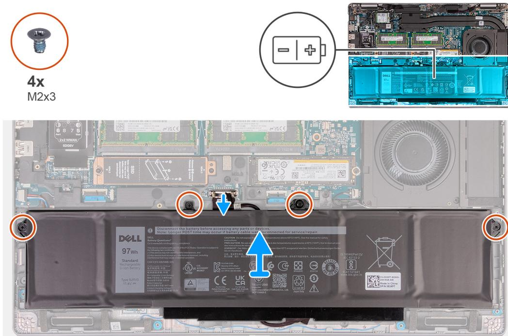
**Figure 38. Removing the battery - 97 Wh**
