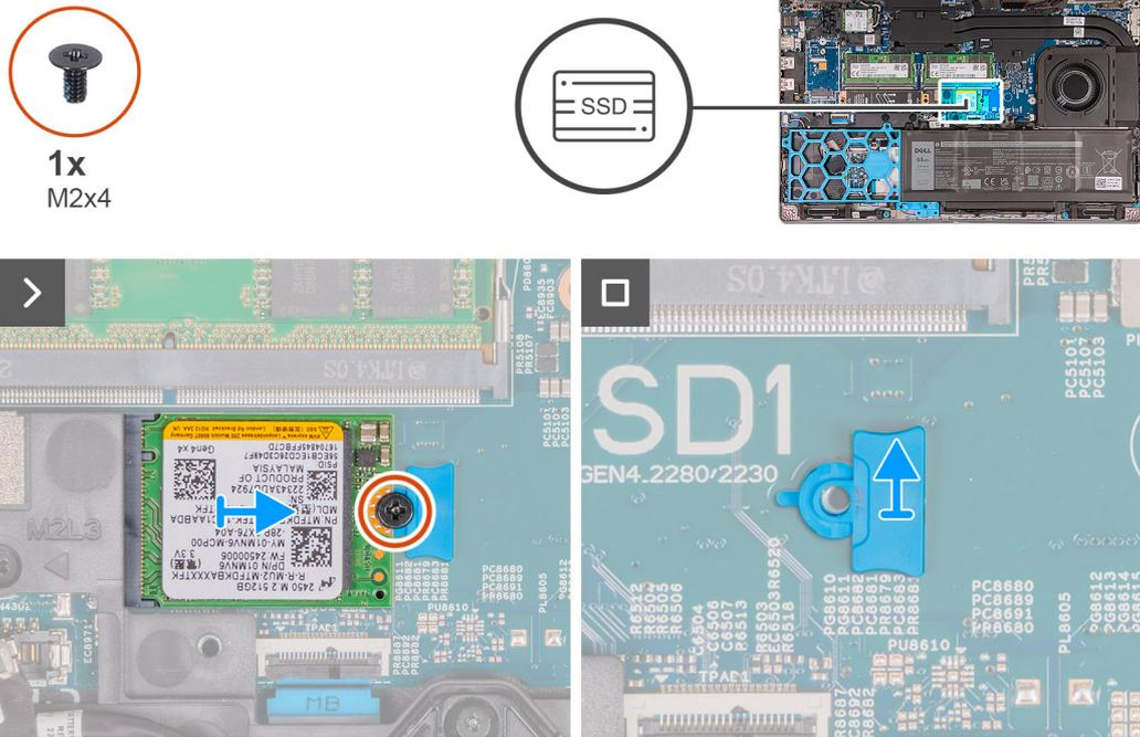
**Figure 27. Removing the M.2 2230 SSD from slot 1**
