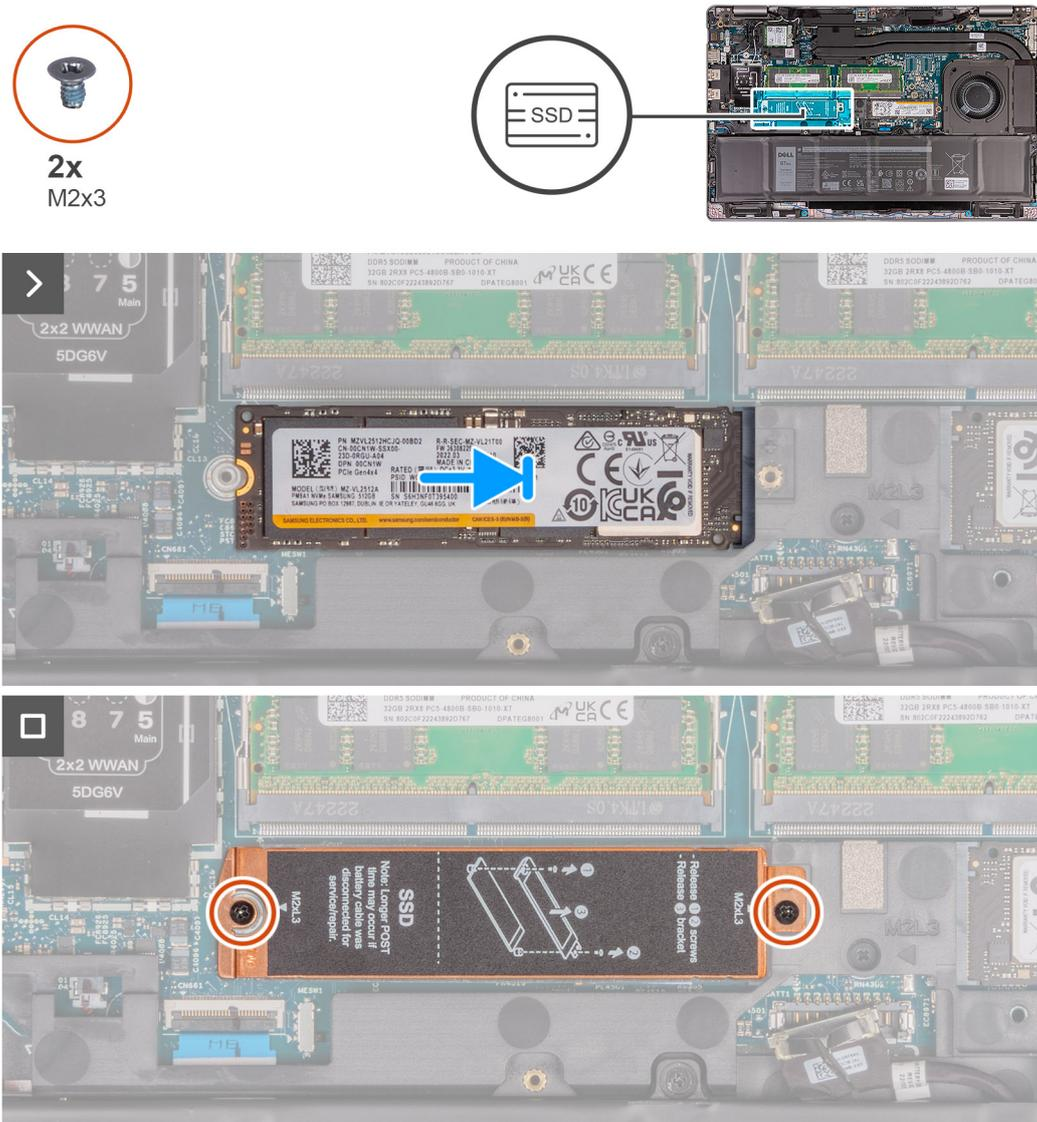
Figure 34. Installing the M.2 2280 SSD in slot 2
