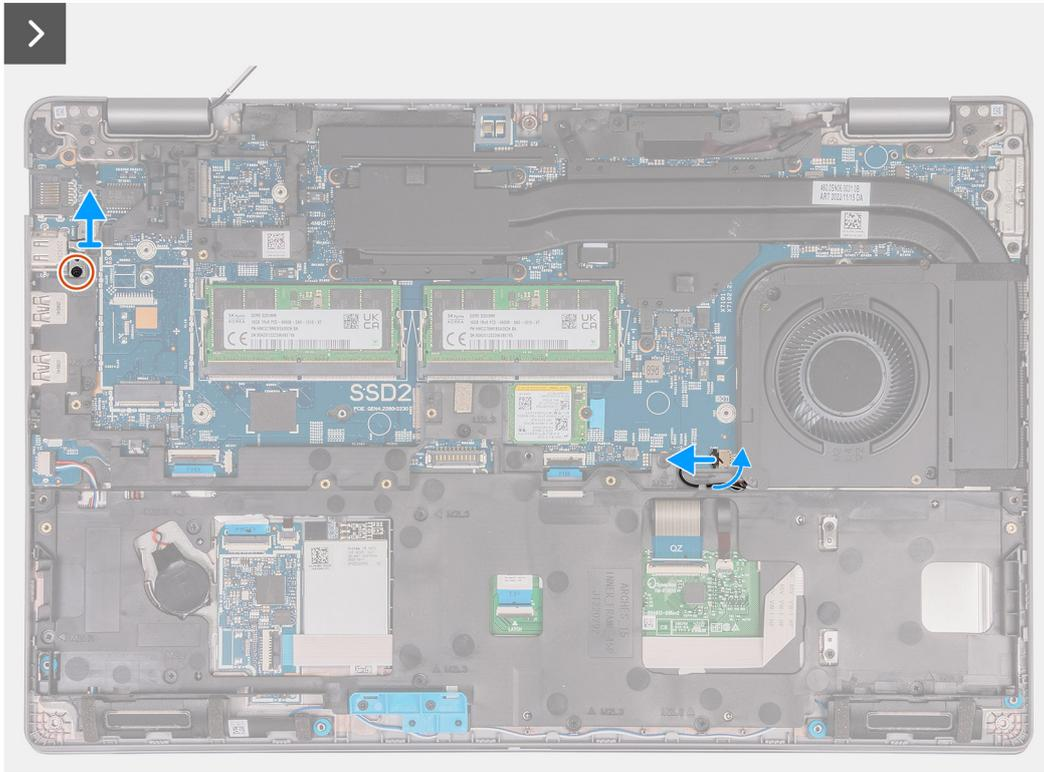
**Figure 41. Removing the assembly-inner frame**
