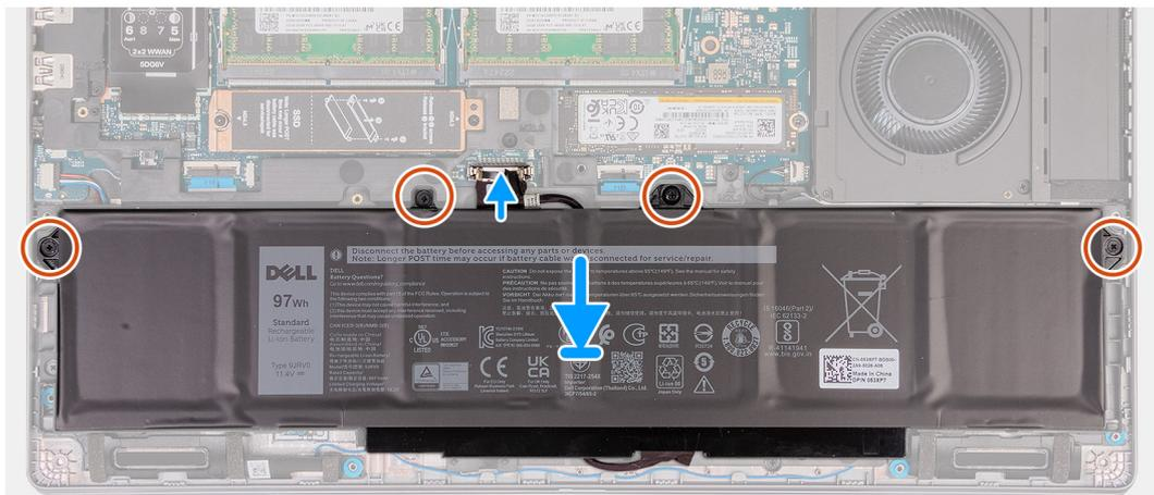
**Figure 40. Installing the 97 Wh battery**
