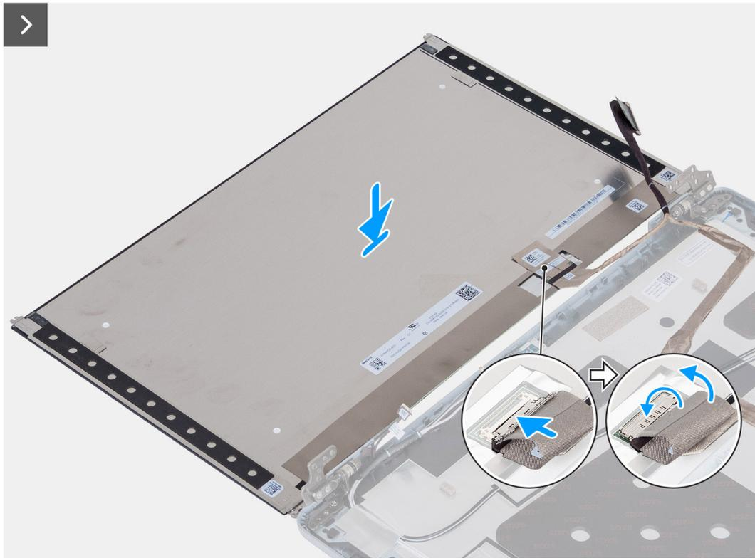
Figure 85. Installing the display panel
