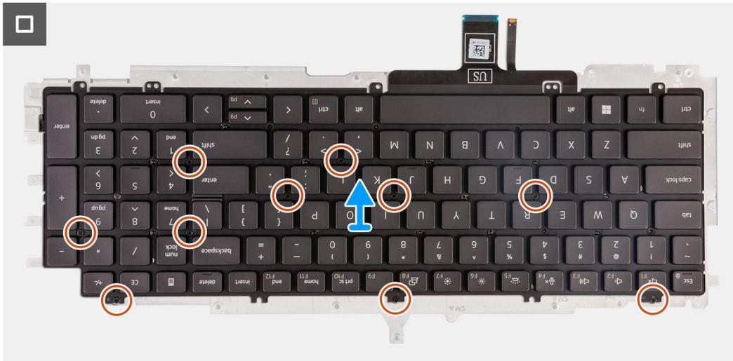
Figure 70. Removing the keyboard
