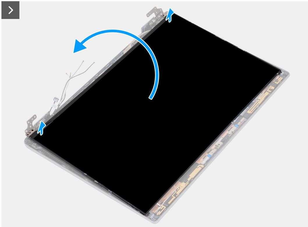
Figure 81. Removing the display panel
