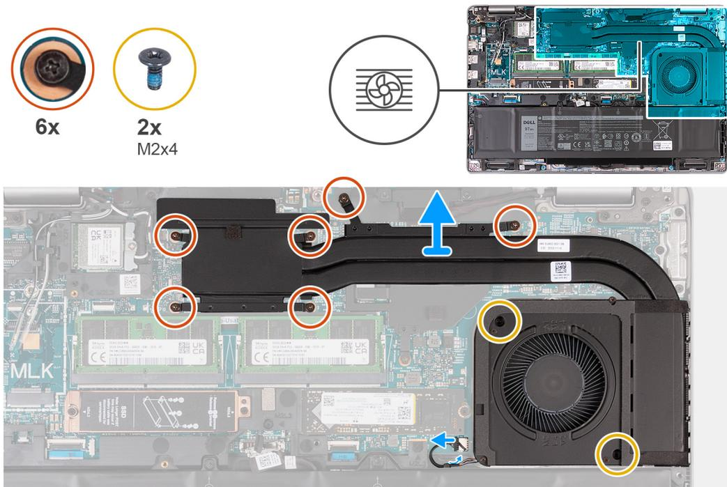
**Figure 52. Removing the heat sink (Discrete GPU)**
