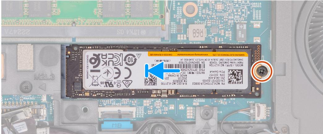
**Figure 30. Installing the M.2 2280 SSD in slot 1**
