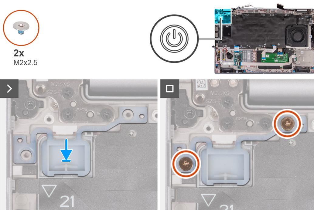
**Figure 66. Installing the power button**
