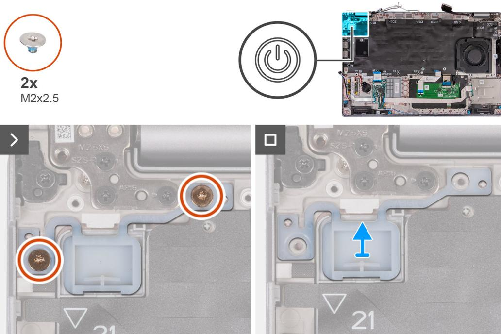
**Figure 65. Removing the power button**
