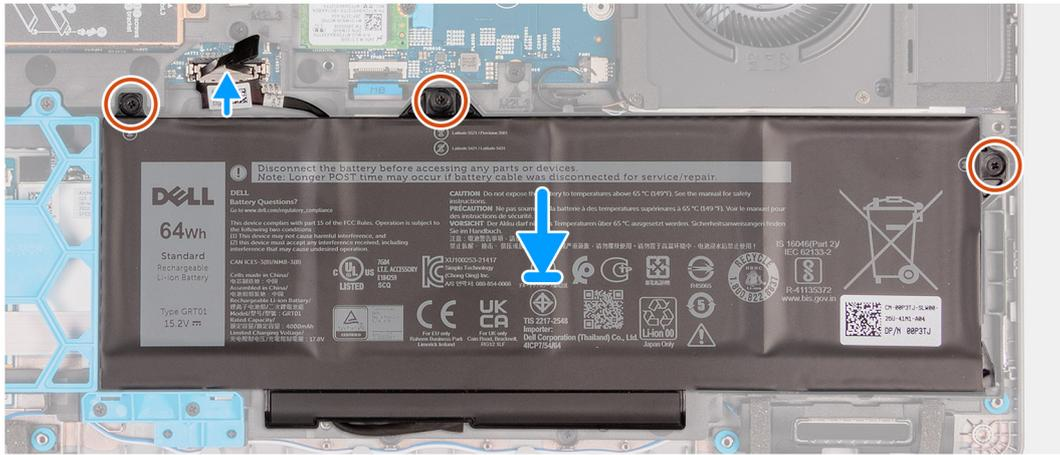
**Figure 39. Installing the 64 Wh battery**
