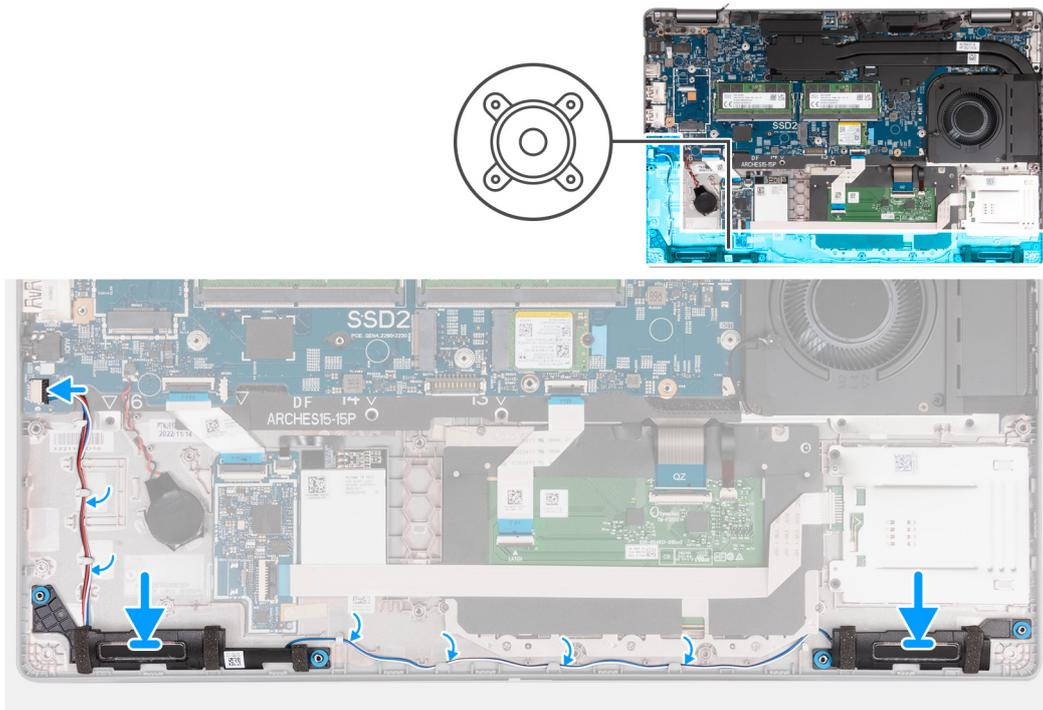
**Figure 48. Installing the speakers**
