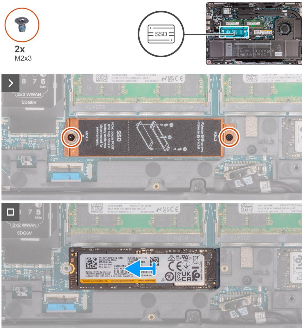
**Figure 33. Removing the M.2 2280 SSD from slot 2**
