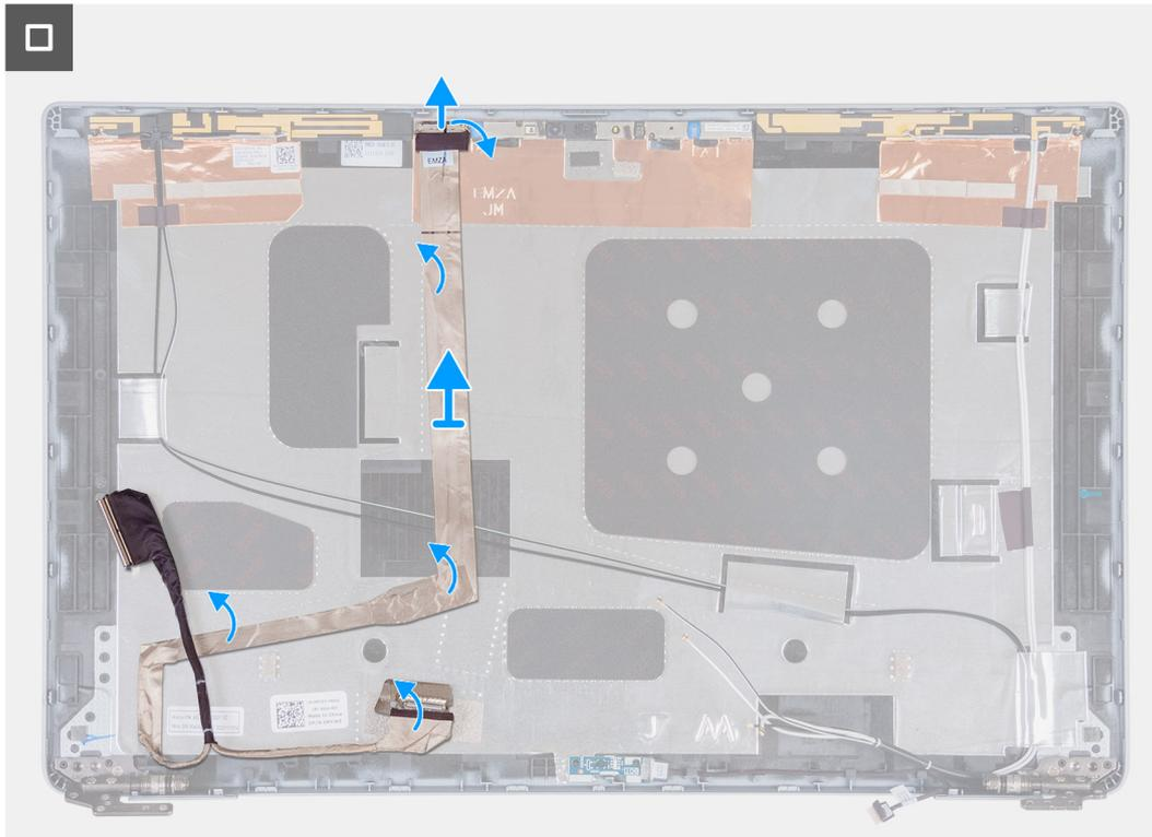
**Figure 94. Removing the display cable**
