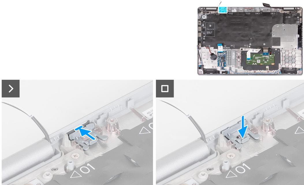
Figure 101. Installing the dummy SIM-card slot filler
