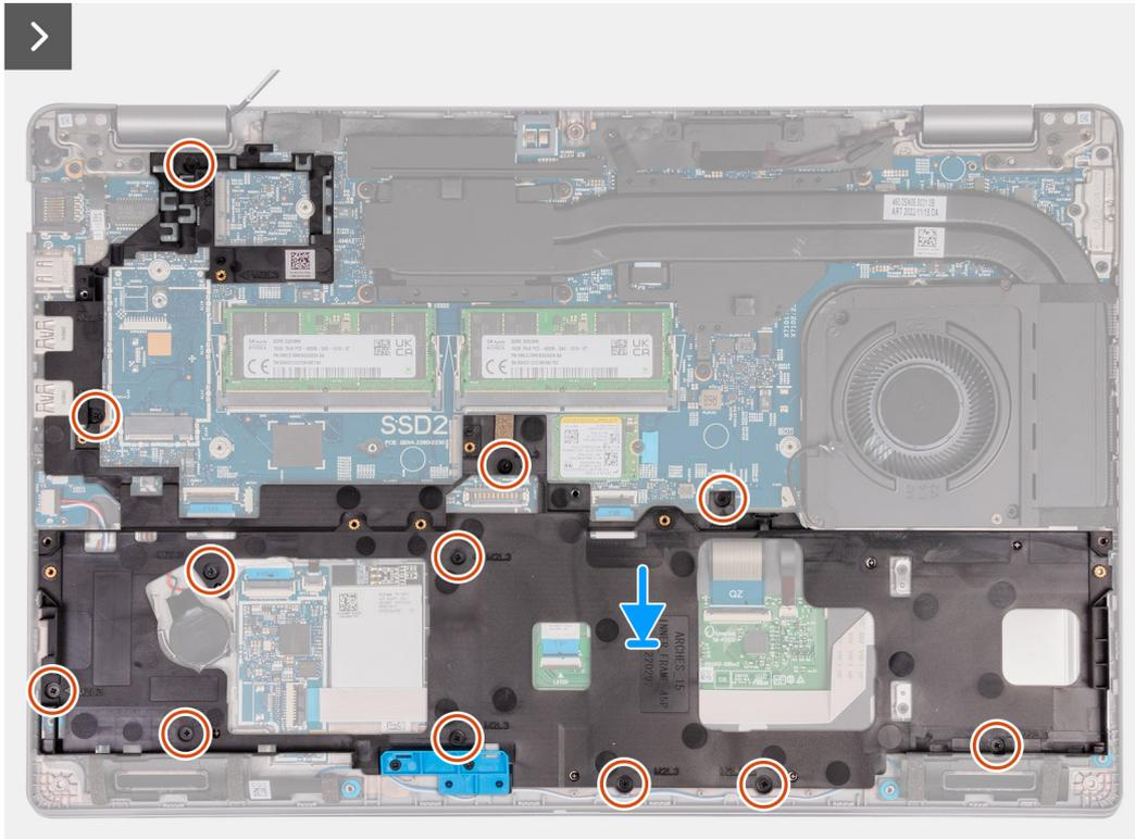
Figure 43. Installing the assembly-inner frame
