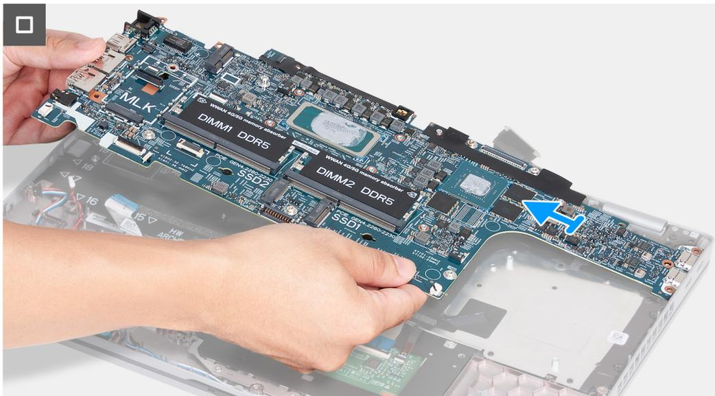
Figure 60. Removing the system board
