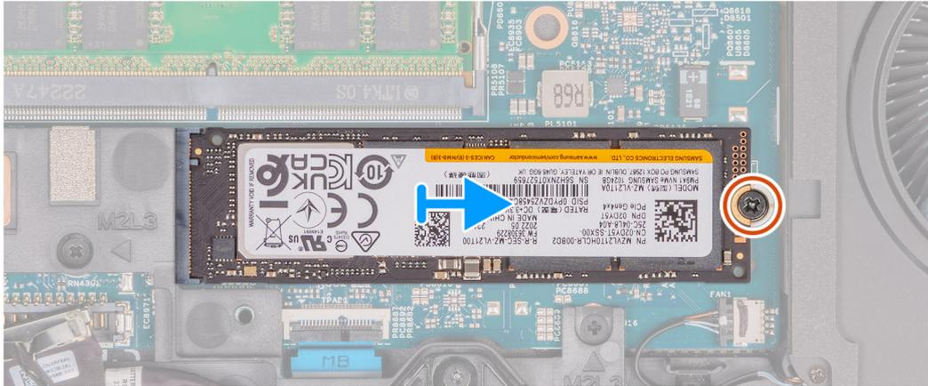
**Figure 29. Removing the M.2 2280 SSD from slot 1**
