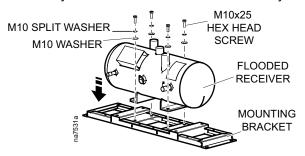
3. Attach the receiver to the side of the ACCU30X unit and connect the cable conduit.
