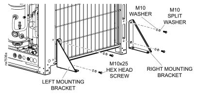
4. Attach the receiver to the mounting brackets and connect the cable conduit. NOTE: The cable conduit can be cut to size; use caution to avoid cutting
