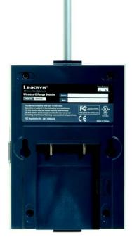
Figure 3-2: Recess for the Power Plate
