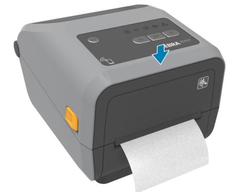
Press down on the front edge of the printer until it locks.
