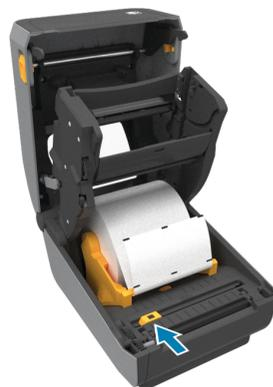
Align the sensor to the edge of the roll for marked labels.
