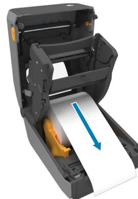
Pull the end of the roll past the front edge of the printer.
