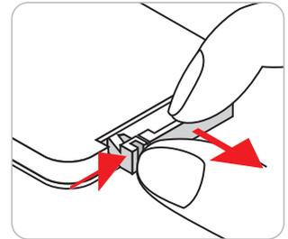
2. Install new battery into the compartment. Remove the old battery and install new one (CR2025). Ensure that the side with a “+” is facing up.
