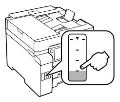
**Note:** The product has a low ink alert system. The accuracy of this system depends on the user refilling the ink tanks correctly. The product cannot directly measure the ink levels in the tanks; instead it estimates the amount of ink remaining by internally monitoring ink usage. The low ink alert system may generate inaccurate messages if the ink tanks are not refilled according to these instructions.
