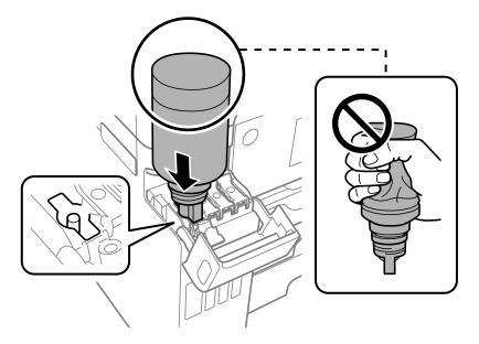
**Note:** Refer to the color-coded sticker on the ink tank unit to identify the color of each tank. Do not force the bottles into position; they are keyed for each color.
