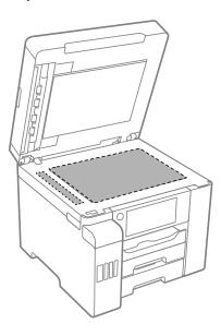
**Note:** If lines appear on the printout or in scanned images, carefully clean the scanner glass on the left.
