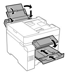
10. Place the printer in a plastic bag and fold it closed.
