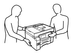
• Avoid tilting the product, placing it vertically, or turning it upside down; otherwise ink may leak. When storing or transporting the printer, place it in a plastic bag and fold it closed.
