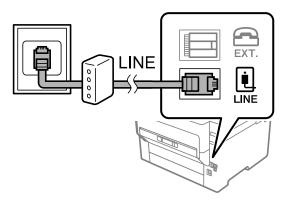
**Note:** If you have a DSL or ISDN connection, you must connect the appropriate DSL filter, or ISDN terminal adapter or router to the wall jack to be able to use the line for faxing or voice calls using your product. Contact your DSL or ISDN provider for the necessary equipment.
