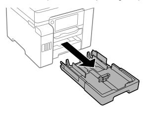
2. Slide the side edge guides outward all the way, then slide the side front edge guide to the paper size you are using.
