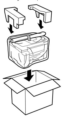
Keep the product level during transportation. If print quality has declined when you print again, clean and align the print head. Make sure you remove the tape securing the print head before using the printer.
