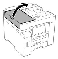
11. Use a soft, dry, lint-free cloth (microfiber is recommended) to clean the rollers and the interior of the ADF.
