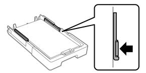
**Note:** Make sure the paper fits beneath the arrow mark inside the edge guides.
