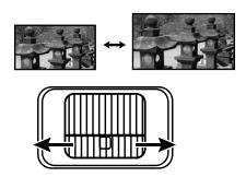
To improve the clarity of the image, rotate the Focus Ring.
