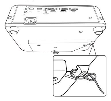
**NOTE:** The security slot can also be used as a safety anchor if the projector is mounted to the ceiling.
