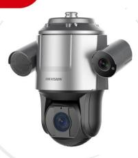
The smart-linkage PTZ camera adopts an all-in-one design with two camera channels, a speaker, and two high-performance GPUs. Integrated with multiple deep learning algorithms for complicated scenes, it provides accurate collection of target feature data, comprehensive data analysis of multiple scenes, and all-around situational perception.
