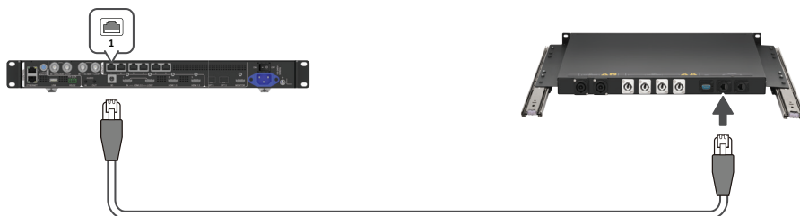
Network Connection between the Power Module and LD-SCB-025 (VX600 Pro) Control Box
